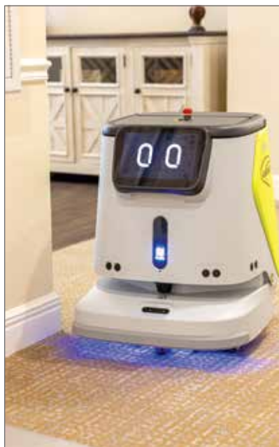
Dirty Harry is the first Pudu Robotics vacuum deployed by Arrow Senior Living that is now being rolled out across the portfolio. The robot manages multi-floor surface cleaning, including vacuuming and water treatment, that fills one part-time position.
